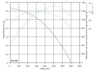
Performance certified is for Installation Type D - ducted inlet, ducted outlet. Speed (RPM) shown is nominal. Performance is based on actual speed of test. Performance ratings do not include the effects of appurtenances (accessories).
