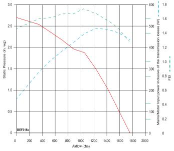
Performance certified is for Installation Type D - ducted inlet, ducted outlet. Speed (RPM) shown is nominal. Performance is based on actual speed of test. Performance ratings do not include the effects of appurtenances (accessories).
