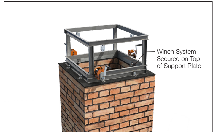
Fig 12-6: Winch System Installed
