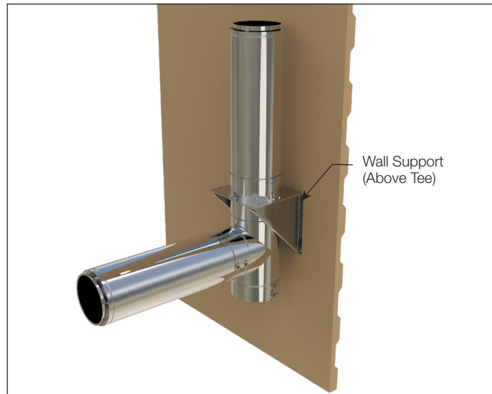
Fig 7-11: Tee Support Example
